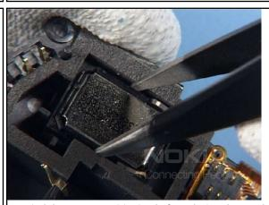
12. Mind the correct positioning before placing the speakers into the CHASSIS.
