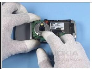
44. Remove the protective film and close the shutter.
