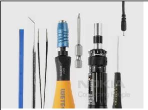
1. Needed tools: SS-93, the dental pick, metal tweezers, a bit holder with a Torx plus size 6 bit, a torque driver, a straight bladed screwdriver and a DC plug.
