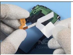
2. Remove the protective film from the 1UJ FLASH MODULE.
