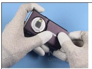
3. Unlock and remove the BATTERY COVER.
