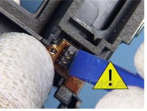
6. Do not bend the connector springs while pushing down.
