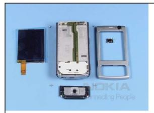
21. The disassembly procedure is now complete.
