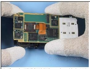
19. Lift up the LIGHT SWAP PWB together with the MAIN CAMERA.
