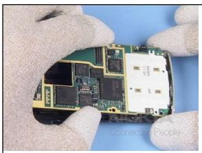
19. Insert the PWB into the CHASSIS, beginning from the bottom.
