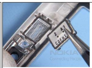
20. ...and must be replaced when reassemble.
